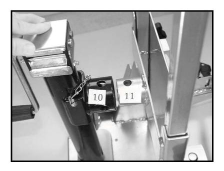
Attach jack (part #10) to cylindrical steel piece (part #11) welded on main stand (part #2) using hitch pin attached to jack (part #10).
