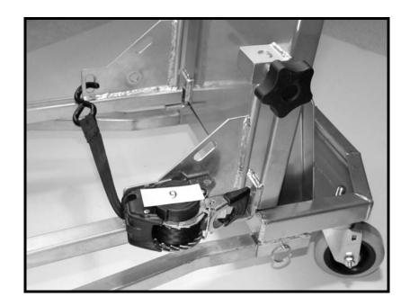
Attach the retractable ratchet strap (part #9) to either side of one lifting arm (part #7) with bolt, washer, and nut in the bag supplied with the ratchet strap. The bolt should insert from the frame side into the washer and nut set inside the ratchet. You may find it easier to mount the strap prior to inserting the lifting arm into slotted hole.
