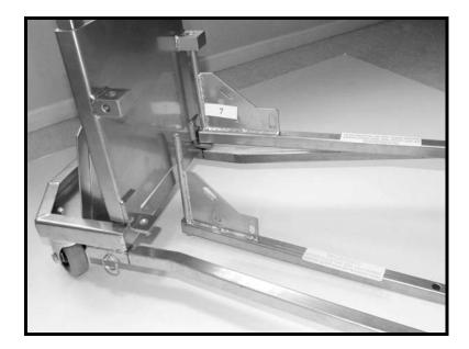
Attach the 2 lifting arms (part #7) with warning labels facing up into slotted holes on each side of main stand (part #2) and drop into place.
