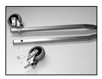
Attach the two 4" front casters with longer bolts (part #3) to bottom legs with slight bend (part #4). The casters are attached with washers and nuts provided in the plastic bag. Attach wheels so that when the next step is done, shown in Step 3, legs will bend to the *outside*.
