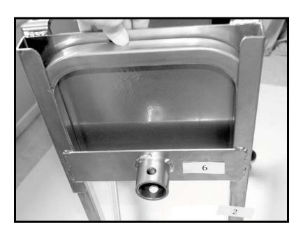
Slide guide plate (part #6) over and down onto main stand (part #2). **CAUTION – avoid pinched fingers!**
