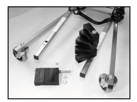
Attach 5 grey "fingers" with bolt provided in plastic bag on each side (part #12). Insert bolt through fingers and attach/tighten one nut. Insert through hole in lifting arm (part #7) and add one washer and nut, then tighten. Do this on each side.
