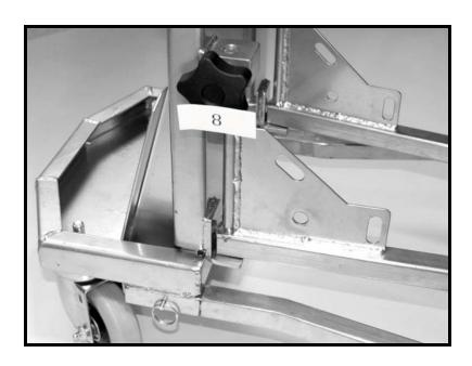
Screw in the two star shaped jib knobs (part #8) to threaded holes to secure the arms.
