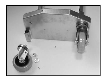
Attach the two 4" rear casters with shorter bolts (part #1) to the main stand (part #2). The casters are attached with washers and nuts provided in the plastic bag.
