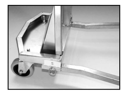
Legs (part #4) attach to main stand (part #2) with two hitch pins provided (part #5). *Note that legs spread outward once mounted.*
